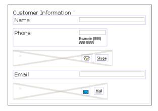
The shaded diagonal lines across two of the panes in this form indicate that the **Visible** property of those panes is initially cleared, or set to false.
