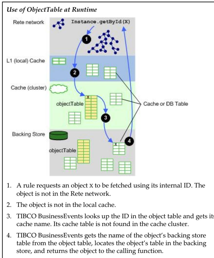
Note that if the object table is not preloaded with the entry for object *X*, then an additional processing step is required, to load the object table in the cache for that object's entry.
