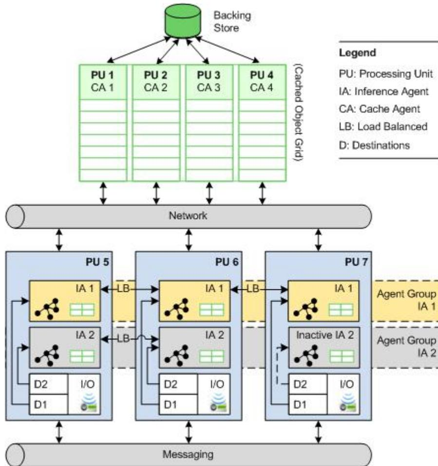
The drawing illustrates one possible configuration, and assumes destinations that are JMS queues using basic load balancing (Content-aware load balancing is also available. See [Load Balancing](#)).
