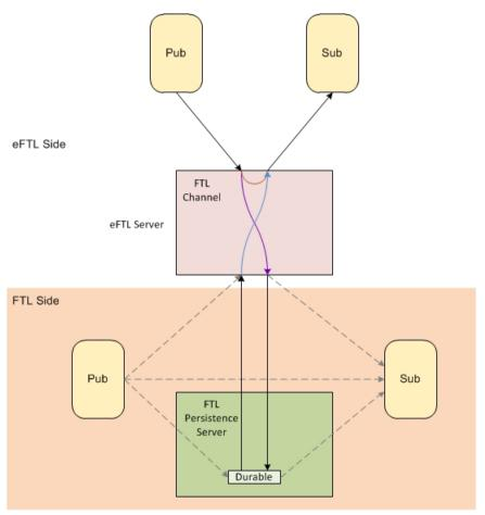
Gray dashed arrows in the diagram indicate that this arrangement does not depend on FTL publishers and subscribers. They need not be present. That is, eFTL applications can use the FTL persistence feature even if they do not communicate with other FTL applications.
