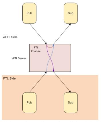
The diagram shows applications that publish and subscribe. Applications at the top connect to the FTL channel using the TIBCO eFTL API, while those at the bottom communicate using TIBCO FTL transports. The channel forwards messages among them in three ways:
