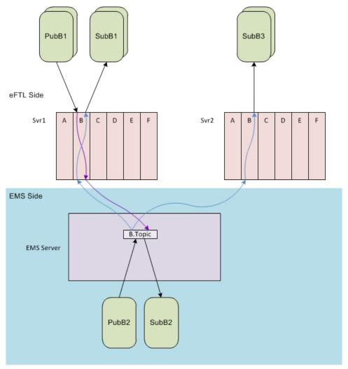
The diagram illustrates a cluster of two eFTL server processes. The purple arrow indicates that when PubB1 sends a message, Svr1 translates it and forwards it the EMS server. The EMS server forwards it in two directions:
