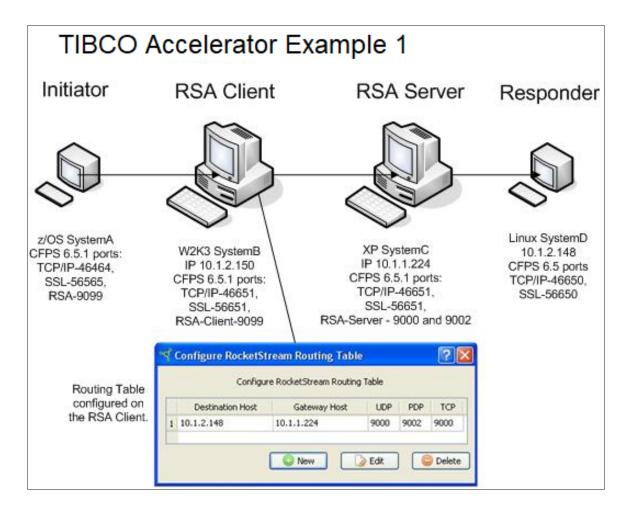
This figure demonstrates sending a file from a Platform Server for z/OS (system A) to a Platform Server for Linux (system D). These two servers do not contain the TIBCO Accelerator technology; therefore, they must forward the data to a Platform Server for Windows that runs the TIBCO Accelerator service. See TIBCO® Managed File Transfer Platform Server for Windows User's Guide for more information on configuring TIBCO Accelerator on a Windows server.
