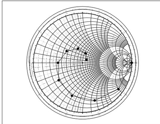
In the Smith–impedance plot, the  $x$  values are resistance data and the  $y$  values are reactance data.
