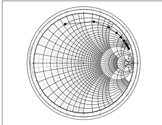
In the Smith-circle plot, the  $x$  values, which must be positive, specify the distance from the center of the Smith plot to the center of the circle you want to draw. The  $y$  values are angles, measured clockwise from the horizontal. The  $z$  values are radii and must also be positive.
