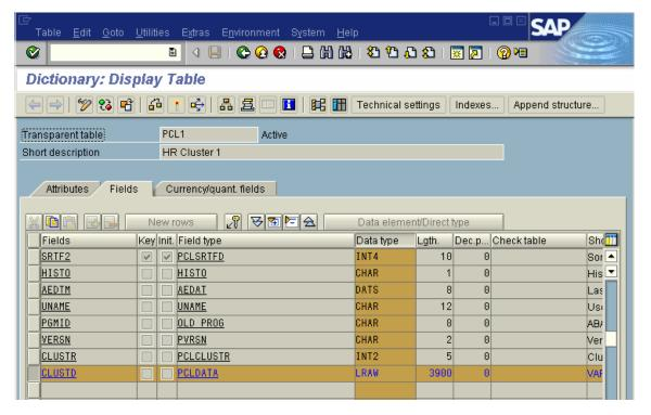
Because SAP is unable to provide TDV access to RAW columns or columns of this length, administrators must write custom BAPIs to expose their data. TDV can then access the custom functions like any other resource.
