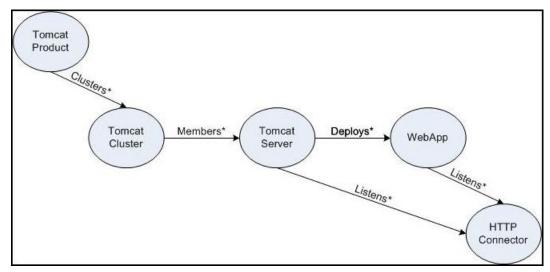
This example does not correspond exactly to the sample Tomcat agent. To illustrate a wider range of concept types, this example explicitly models the cluster and HTTP connector as managed objects. The sample code implements a simpler model, which omits these entities.
