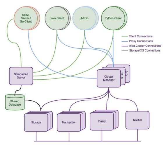
The diagram depicts a variety of components and other processes that communicate within a Graph Database ecosystem. (To simplify the diagram, the diagram omits redundant connections to duplicate processes).
