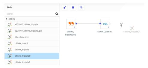
Once you drop the existing target onto the data flow canvas, it will be represented by the database-specific icon and will have the load options specified when the target was first created, with the default merge option. You can edit the options for merging the data into the target by right-clicking the target and clicking *Load Options*. You can also edit the merge expressions and conditions by right-clicking the target and clicking *Merge Editor*.
