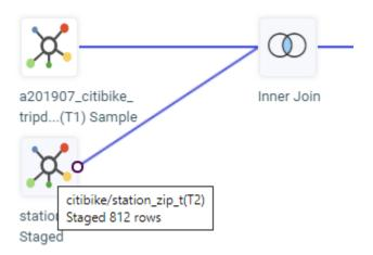
By default, sources are staged as DATREC files. However, you can configure them to be staged in the same relational data source as the target using the SMPL\_ETL\_TRG\_DBMS parameter in Settings for Web Console Preferences on the Workspace page Settings menu.
