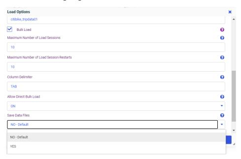
The default value, *No*, deletes intermediate \*.ftm files from the directory for temporary files (for example, edatemp) after the corresponding portion of data is successfully committed to the target table during the Bulk Load Flow execution.
